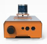
InDro Commander builds on the benefits of a common operating system such as ROS, by bringing a standard suite of sensors and systems (camera, GPS, IMU, Computers Power distribution, communications, 4/5G) that can all be simply, but powerfully integrated onto any ground robot.
