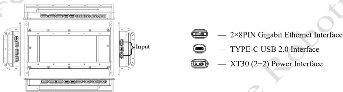
B1 Users' Extende Dock - System Frame Diagram (Structure Top View) is shown in the figure:
