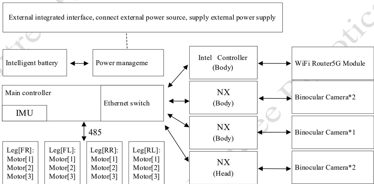
**Hardware interface:** Interface is provided in the back cover of B1 for users, through which developers can directly access to Mini PC and NX controller. The hardware interface is shown in the figure, in which the head NX controller does not open the Type-C and HDMI interface.
