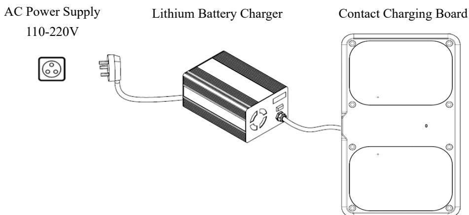
2) Charging: When using the contact charger to charge, first use the remote control to control the robot to lie down, so that the bottom 2 charging electrodes of the B1 robot are in contact with the charging plate 2 charging electrodes to achieve charging, and the button on the lithium battery charger can switch between fast charging and slow charging. When the charge is full, the charger is automatically disconnected from the battery.
