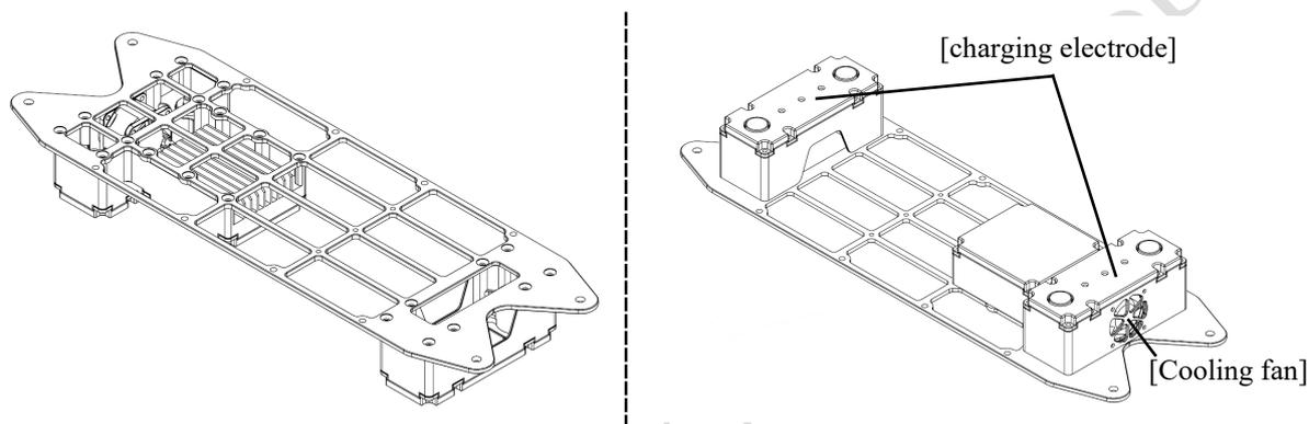
**B1-Contact Charger parts list:** The B1-Contact Charger consists of a lithium battery charger and a contact charging plate.
