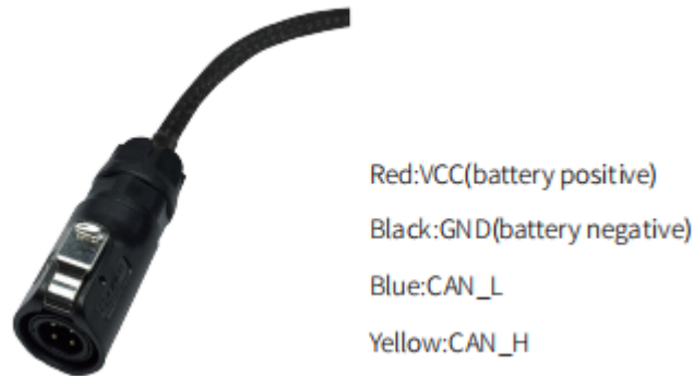
Figure 3.2 Schematic Diagram of Aviation Male Plug
