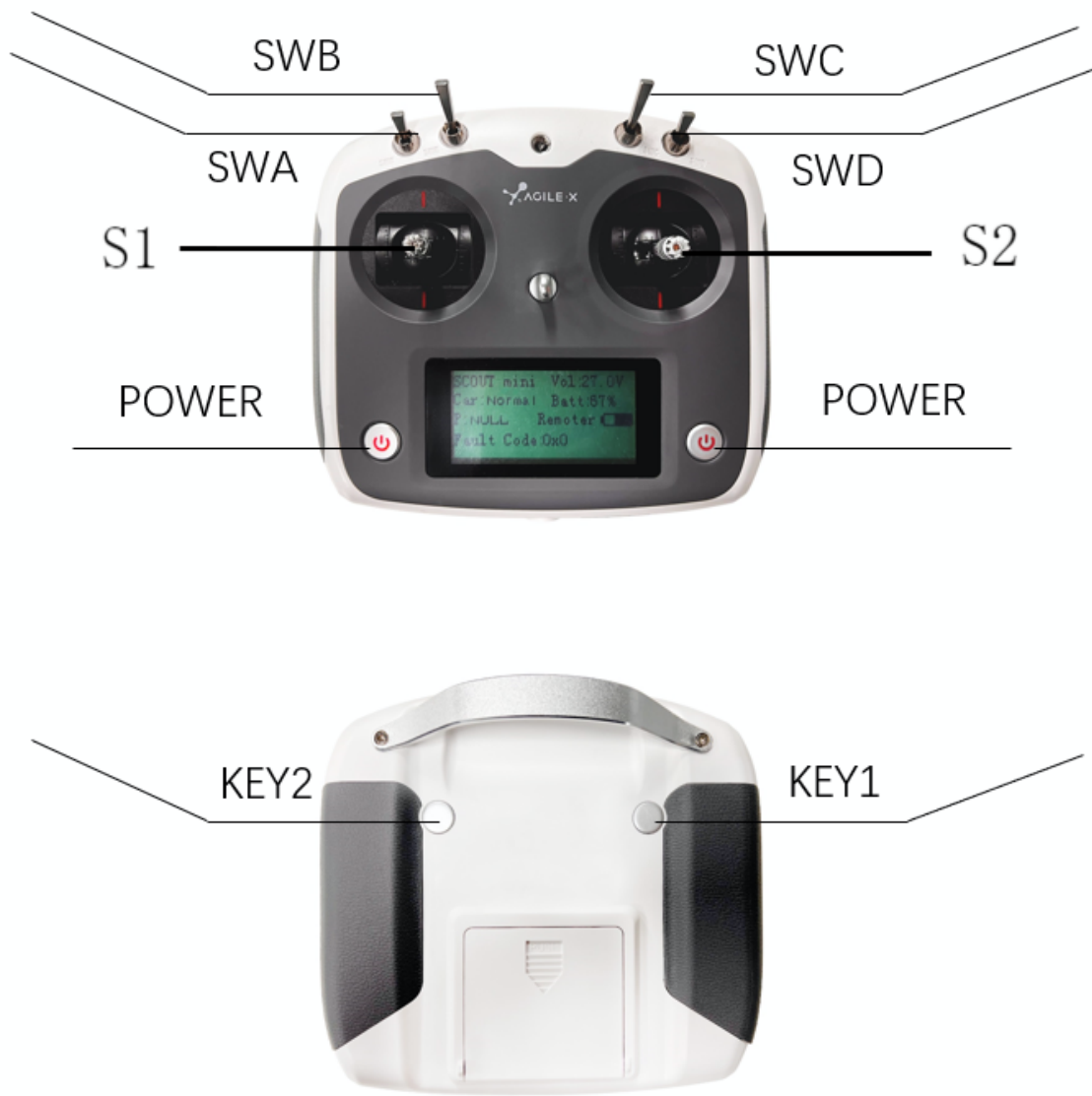
Figure 2.3 Schematic diagram of the FS remote control buttons
