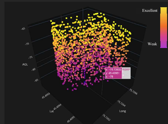
Fig. 19 RSRP mapping in the sky, like RSSI, gets better with higher AGL
